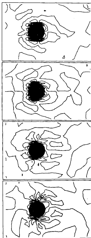
Fig. 4a Streamlines around a circular cylinder ( Re = 10^3 , t = 0.2, 2.0, 3.4, 6.8 ).
